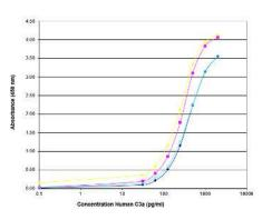
IA: Three different batches tested in a sandwich ELISA to determine the specificity of HM2074. HM2074 was used as detection antibody.
