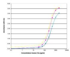
IA: Three different batches tested in a sandwich ELISA to determine the specificity of HM2074. HM2074 was used as detection antibody.
