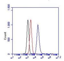
FC: detection of Galectin-3 in Huvec cells. Red, black and blue line represent the isotype control, cells only and HM2186 with a concentration of 10  $\mu$ g/ml, respectively.
